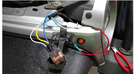
A work in progress. I like to use <u>shrink tube butt connectors</u>. (I haven't shrunk them yet here.)
