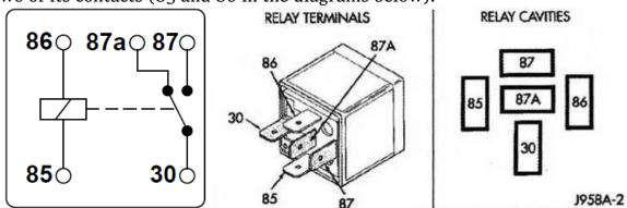
Notice how 30 is connected to 87A in the image on the left. This is its position when no current flows through 85-86. It switches to 87 when current flows through 85-86.
