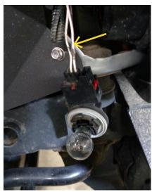
filament, instead it acts as a low resistance path to ground. If you turn off your marker lights and activate your turn signal, current flows backwards through the side marker light as well as
