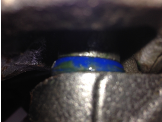
Cap seated against u-joint, with no gap
