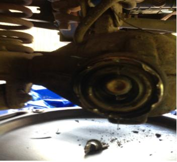
The old seal didn't want to budge. Shocking, right? So I hammered the edges in. V-e-r-y carefully
