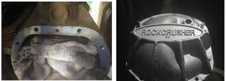
When it comes to prepping for sealant, you can't be to anal. Clean and prep the surface right the first time, or clean and prep it when you go back and do it the second time. I use a wire wheel on the surface, and stuff rags into the diff to keep crap out. This also sops up the pool of old diff fluid. The final step was to rattle can my diff cover, prior to bolting it back on. With an appropriate sealant, of course
