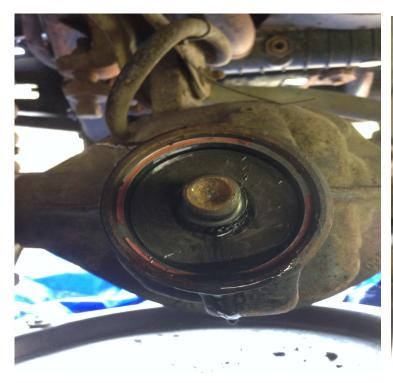
Yoke is out. See that orange on the inside perimeter? It needs to come out. Use a screwdriver and slowly scrape it off. Like you're shaving. It peels right off
