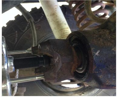
X marks the spot. I lined them up for reassembly and you can't see it now but I also marked the retaining nut so I know how much to tighten it
